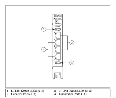
Figure 1-2. Front Panel of the NI PXI-8310 Expansion Card
